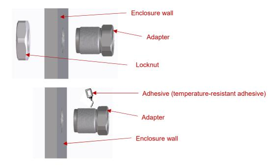
Fixing details for application with vibrations:
