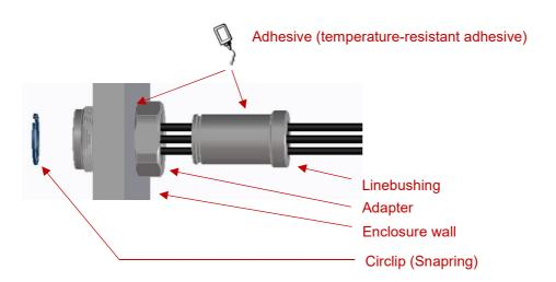
Fixing details for application with vibrations:
